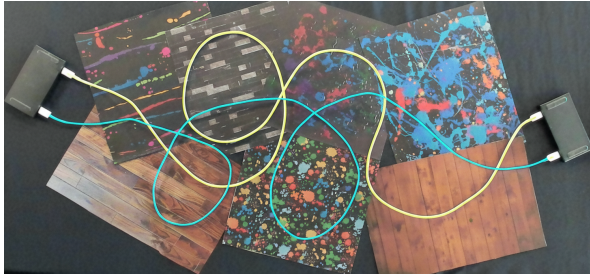
Fig. 12: One successful result by TRACE (100% of cable length correctly traced) on a workspace with highly varied, patterned background clutter.
